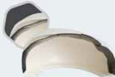
Traditional toe-protection and toe-cap gluing
