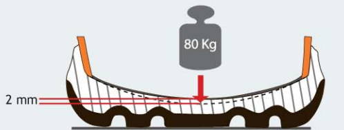
Normal sole with only 2 mm compression
